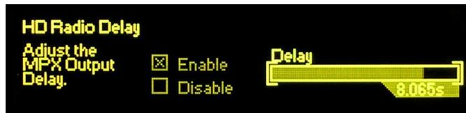
Now *turn* the knob to set the time to 8 seconds and *push* it to activate the setting.
