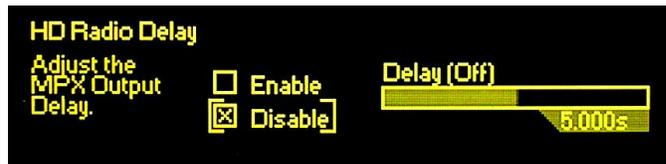
HD Radio delay may be set in 1 millisecond increments anywhere between 1ms and 9.999 seconds. This is a much wider range than required, but anticipates welcome improvements in the encoding/decoding process of the HD Radio system.
